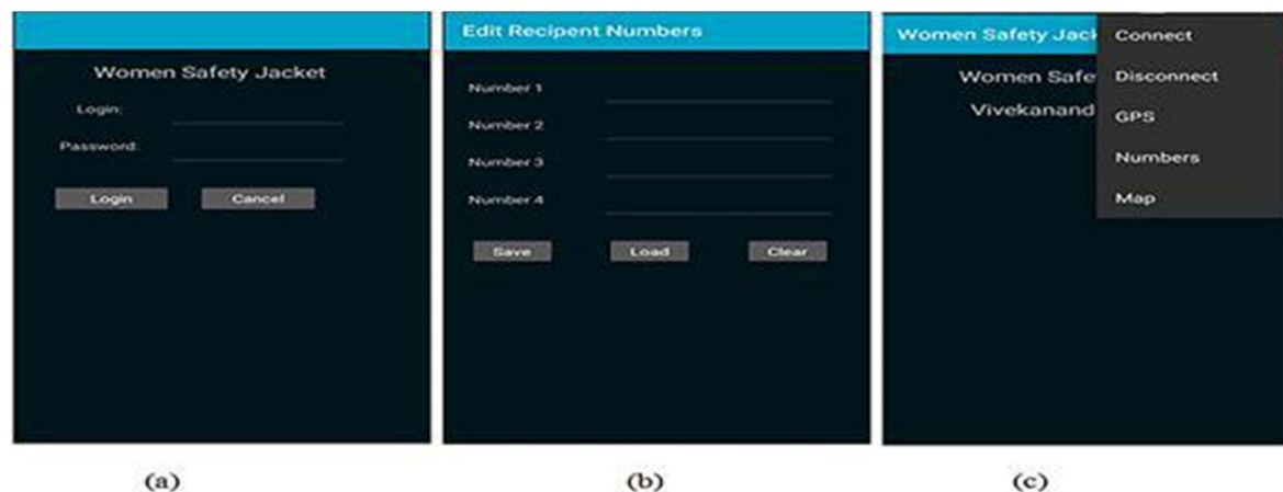
Fig.2 (a). Login & password entry (b). Entry of predefined numbers (c). Connection & disconnection of Bluetooth via app
