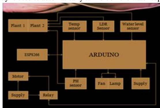
Figure 3: Block diagram of automated hydroponic farm.
