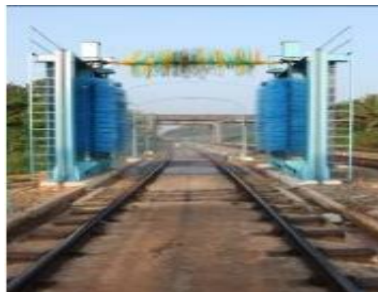
Fig. 2 Soap solution spray and first brush
