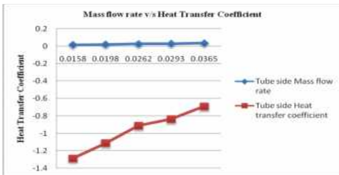
Fig e. Variation of Heat Transfer Coefficient w.r.t Flow rate on the Tube side
