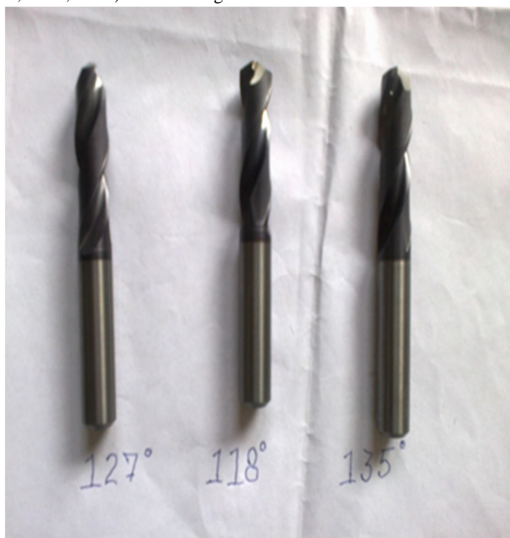
Figure 1: Drill bits having different point angles
