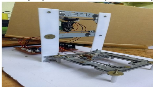
Fig. 10 Mounted X Axis On Y Axis
