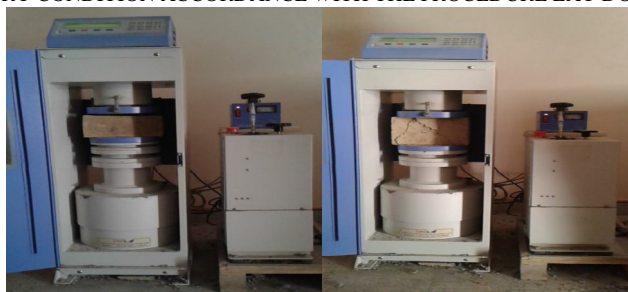
Fig. 4. Adobe blocks under compression
