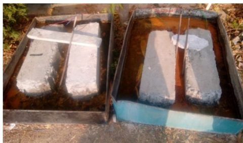
Fig.6 Accelerated corrosion process setup.
