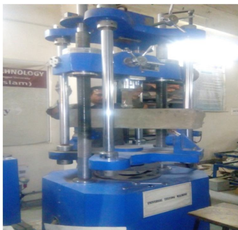
Fig.8 Universal testing machine.
