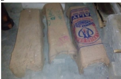
Fig.5 Curing of beams.
