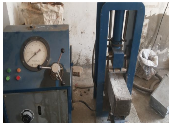
Fig. 6 Flexure strength test
