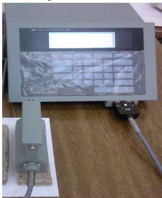
Fig. 6 Thermal conductivity coefficient measurement device
