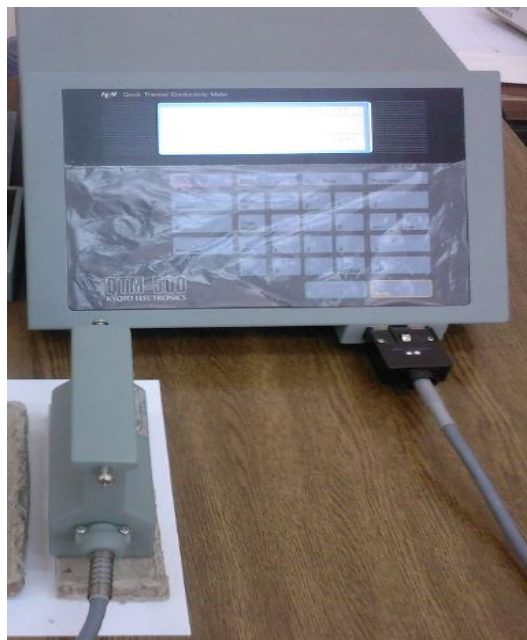
Fig. 6 Thermal conductivity coefficient measurement device
