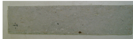
Fig. 4 Trimmed paper-based building specimen
