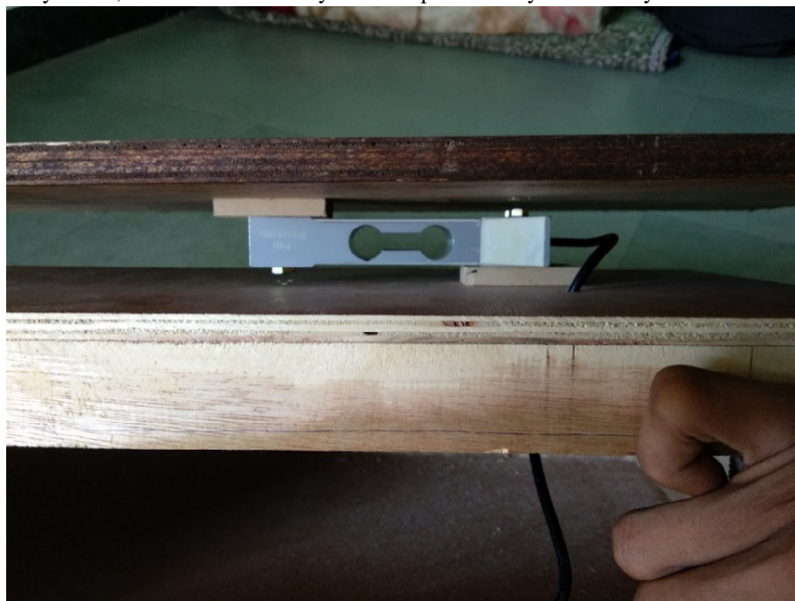
Fig. 9 Load cell mounted on two plates
