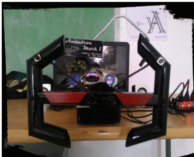
Fig 3:A Close-Up View Of The Steering Wheel, Which Includes Nitro Buttons To Speed Up The Car During Game Play.
