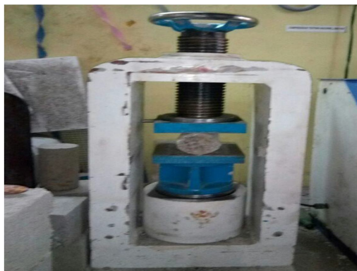
Fig 4a Tested specimen for split tensile
