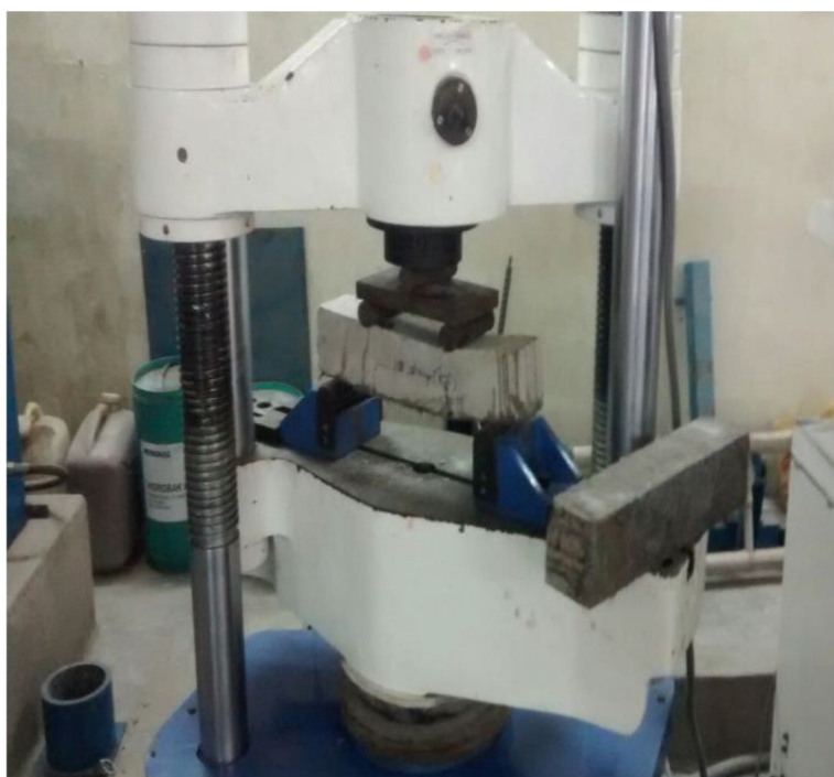
Fig 5a Tested specimen for Flexural strength
