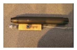
This pen is used to manipulate images on the projected screen. This pen emits Infrared signal which is captured by Wii remote.
