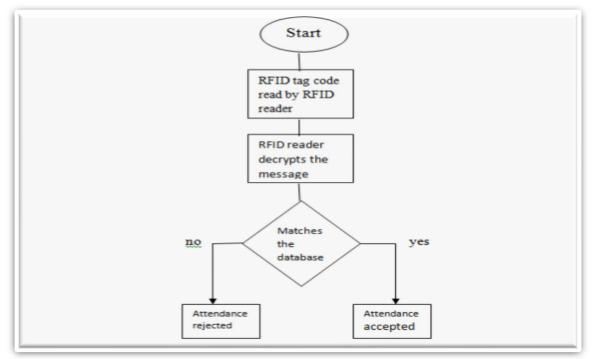
When the system turn on RFID comes in the range and RFID reader transmit the signal to the tags and decrypt the signal. When the authorized code matches with stored information then only attendance has been recorded. If unauthorized card is detected then it will reject that entry.
