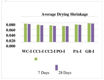
The above chart shows the result for Dry Shrinkage Test results for Concrete Mix Design I. The Test results were carried out on cylinders casted for Curing methods as mentioned earlier. As no standard instrument was available in the college, a new instrument was assembled to carry Drying Shrinkage Test on the Cylinders Casted. The test were carried out on cylinders immediately after initial setting time of concrete and 28 days of effective curing of concrete.
