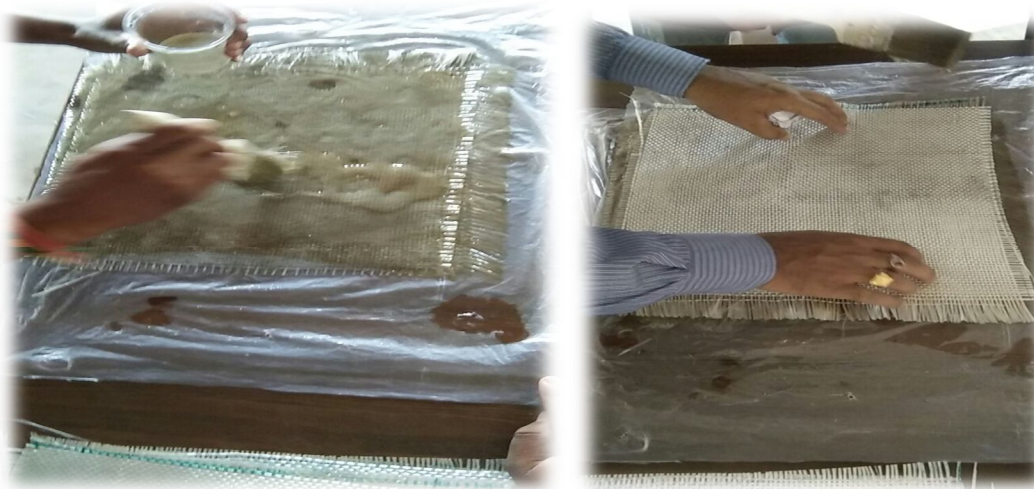
Fig11: Sample preparation by wet hand lay-up process
