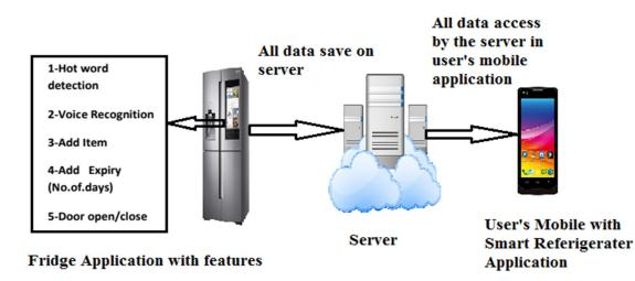
Fig.1 System Architecture Diagram V. WORKING
