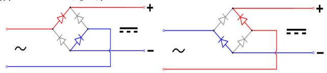
n each case, the upper right output remains positive and lower right output negative. Since this is true whether the input is AC or DC, this circuit not only produces a DC output from an AC input, it can also provide what is sometimes called "reverse polarity protection".
