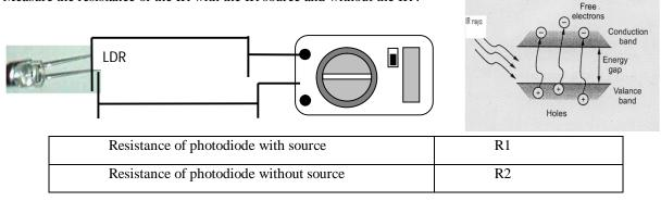
Always  $R_1 < R_2$  We apply a +5 V power supply across the IR receiver. Now if we put the IR source in front of receiver resistance changes. So if the resistance changes the voltage drop across it must also change.
