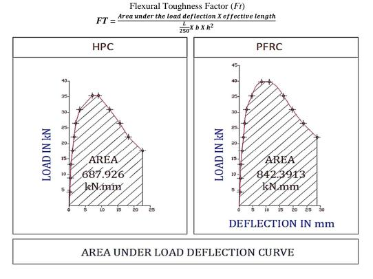
The flexural toughness factor for High Performance Concrete was found to be  $9.5545 \times 10^{-3}$  and that of Fiber reinforced High Performance Concrete was found to be  $11.79 \times 10^{-3}$ . There was an appreciable increase in the flexural toughness factor by the addition of fiber in HPC.
