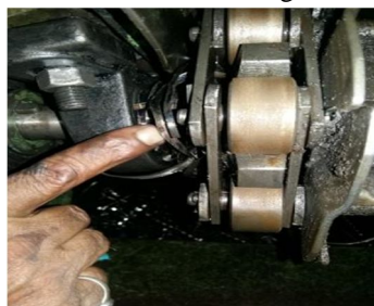
Fig. 6 Chip Stuck on the Bearing Shaft
