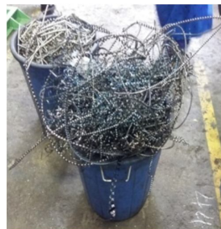
Fig. 8 Chips of Profiling Operation on Wheel Lathe Machine
