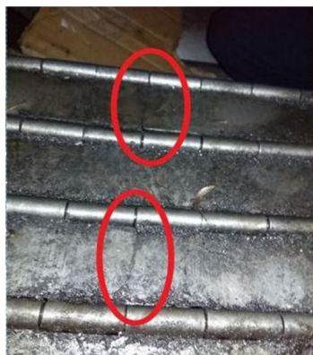
Fig. 13 Sheared Hinge Plate & Bent Hinge Plate
