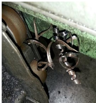
Fig. 7 Chip Stuck Between the Side Links & Roller
