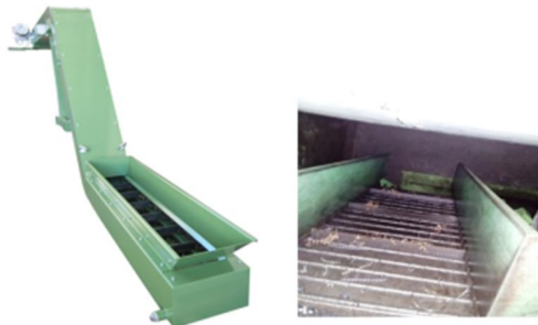
Fig. 1 Hinged- Belt Conveyor
