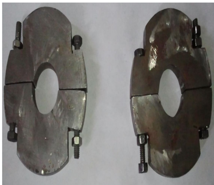
Fig 3.1: Rotor discs having 90 mm outer diameter & thickness 15 mm.
