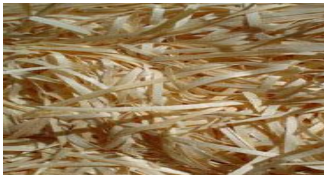
Fig V: Wood Wool Cooling Pad
