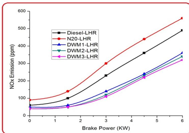
Figure 6.7 Brake power Vs oxides of nitrogen (NO<sub>x</sub>) emission of diesel, N20 biodiesel, and diesel-water emulsion in LHR engine
