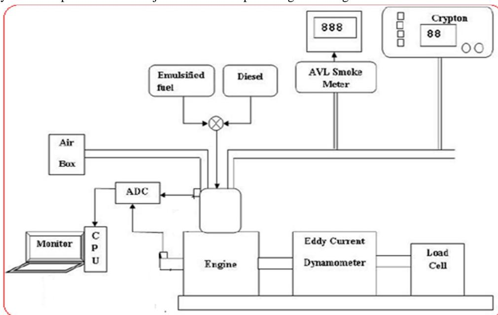
Figure 4.1 Schematic diagram of experimental layout
