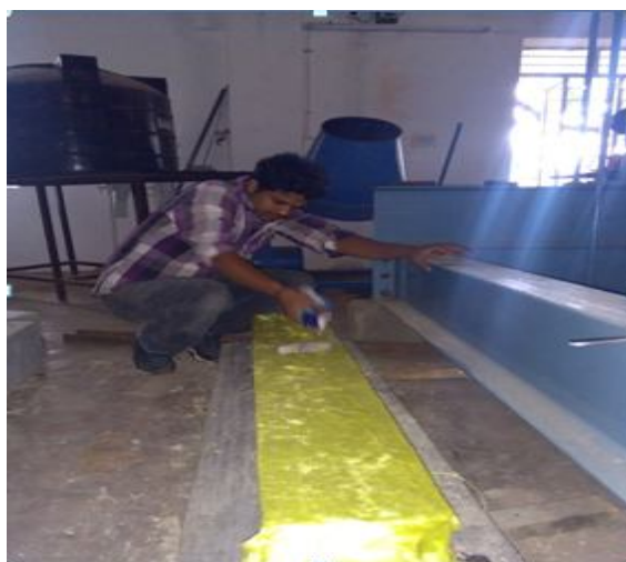
Fig 4: Application of Epoxy and Aramid fibre
