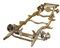
Advantages of this type chassis: it is easy in construction, It is cheaper than other chassis. However, it possess disadvantage since it is a dimensional structure, tensional rigidity is very much lower than other chassis, especially when dealing with vertical loads or dumps.
