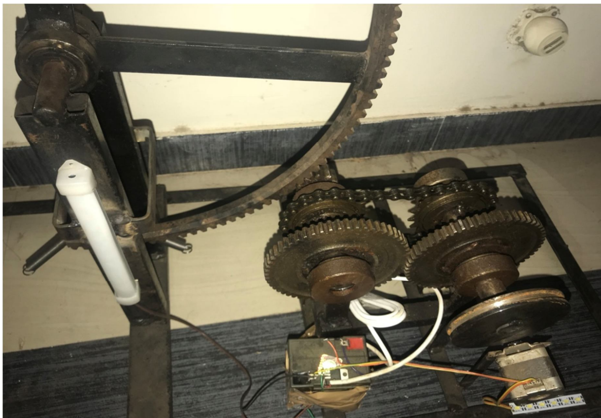
Fig:-3 Uni directional Gear Mechanism used in the design
