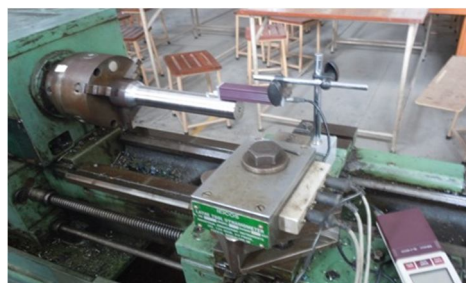
Fig. 2 Measurement of surface roughness
