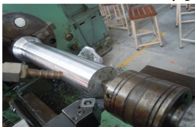
Fig. 1 Coolants used at tip of the tool
