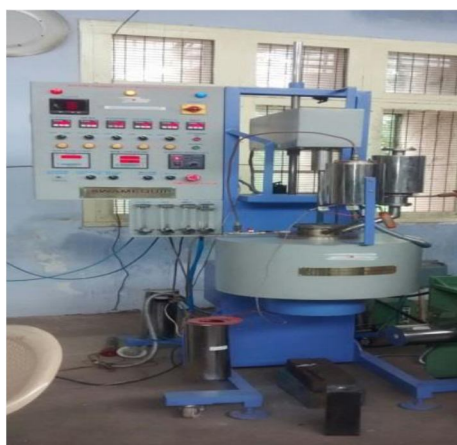
Figure 1 Stir Casting Setup
