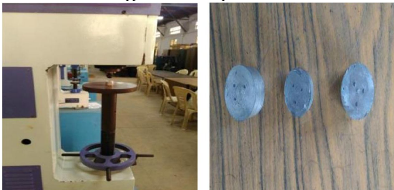
Figure 3 Brinell hardness Tested Specimens
