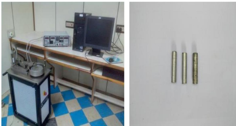
Figure 4 Brinell hardness Tested Specimens
