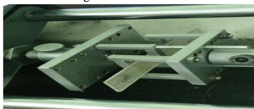
Fig. 5 Bending specimen with fixture
