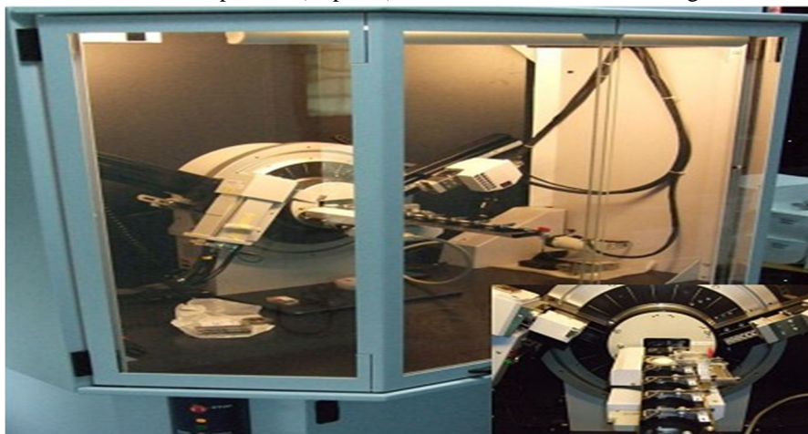
Figure3.8: Bruker Advance XRD
