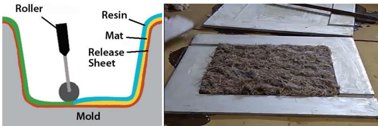
Fig. 3 Fabrication of composite by Hand Layup Technique.
