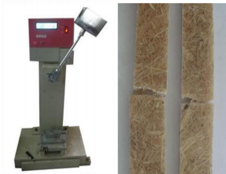
Fig.7. Impact Test Setup and Specimens.
