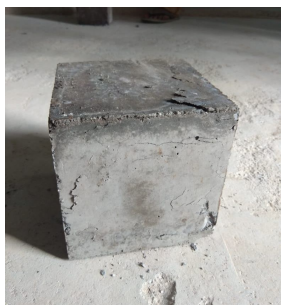
Fig.4 Cube Crack Pattern
