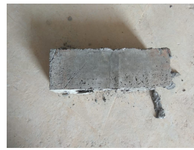
Fig. 6 Prism Crack Pattern
