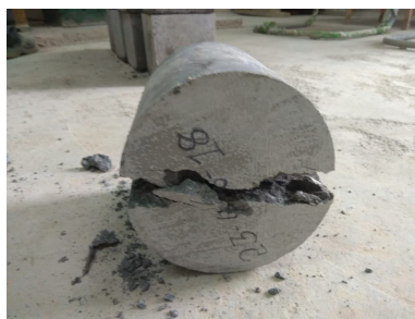
Fig. 5 Cylinder Crack Pattern
