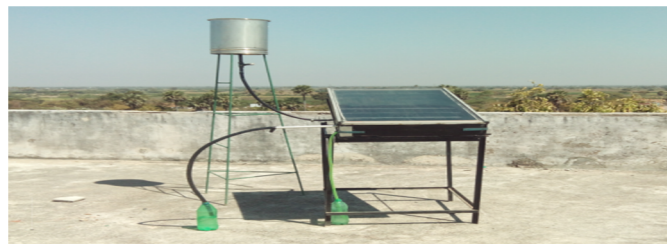
Fig 3 : Experiment setup without parabolic concentrator
