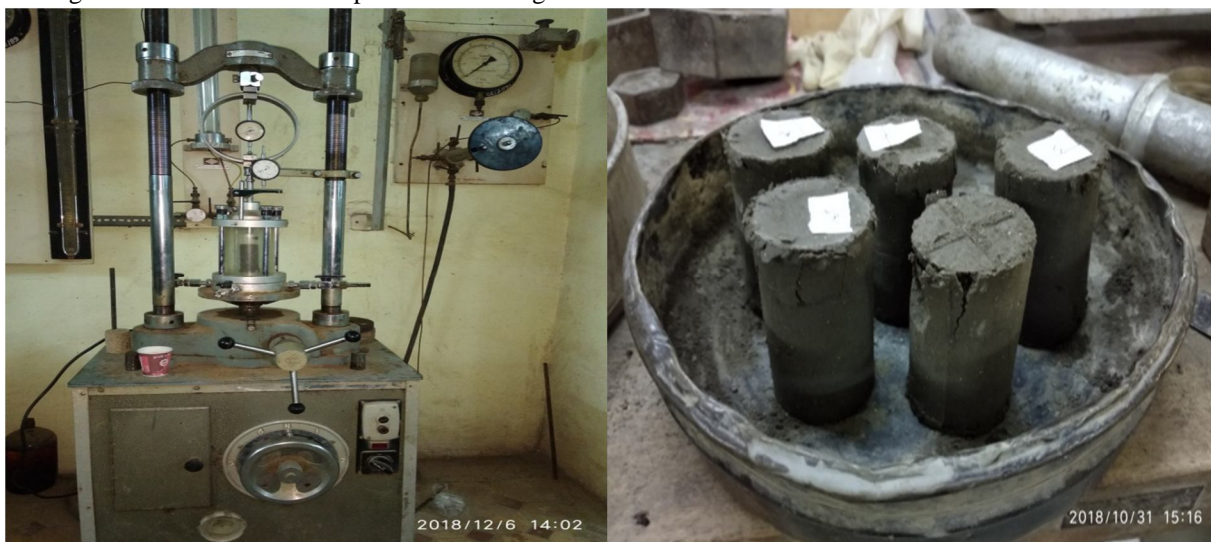
Figure2. Unconfined compressive strength test (UCS)
