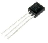
Temperature sensor is a gadget which detects varieties in temperature crosswise over it. LM35 is a fundamental temperature sensor that can be utilized for test reason. It give the readings in centigrade (degree Celsius) since its yield voltage is directly relative to temperature. It utilizes the way that as temperature expands, the voltage crosswise over diode increments at known rate (really the drop crosswise over base-producer intersection of transistor)
