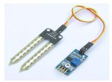
Soil dampness sensors normally allude to sensors that gauge volumetric water content. Another class of sensors measure another property of dampness in soils called water potential. These sensors are usually referred to as soil water potential sensors and include tensiometers and gypsum blocks.
