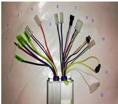
Figure 2: Motor controller
