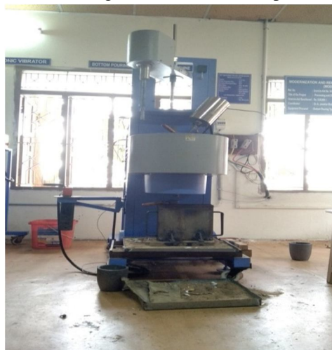
Fig – 1: Bottom pouring stir casting machine
