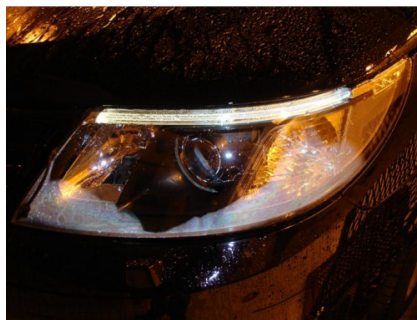
Figure 2 Condensation Has Taken Place on Headlamps
