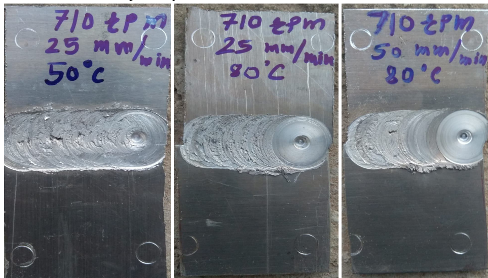
Fig. 4 Welded Plates of 710 rpm
