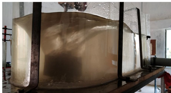
Figure: Working image of gravitation vortex water turbine
