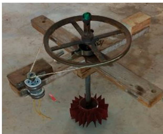
Figure: Blade and dynamo unit
