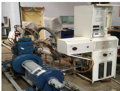
Fig. 6 Computerized variable compression ratio test rig.
