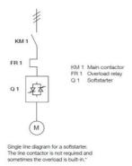
Using a softstarter will reduce the starting current and thereby avoid voltage drops in the network. It will also reduce the starting torque and mechanical stress on the equipment, resulting in reduced need for service and maintenance.
