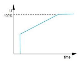
Since the voltage to the motor is reduced during the start, both the current and the torque will also be decreased. In fact, if the voltage is decreased to 50% of the full voltage, the current will be decreased to about 50% of the maximum current at that speed and the torque will be decreased to about 25% of the maximum torque.
