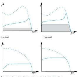
orque and current curves when starting a low loaded motor and fully loaded motor using a softstart
