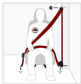
Fig. 2 Safety belt positions & location of end point fixation
