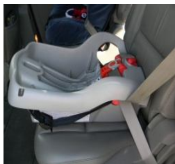
Fastening of CRS to the cars with seat belts
