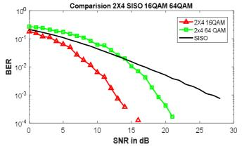
From the figure, it can be concluded that  $2\times4$  16-QAM gives better results compared to other modulation techniques when there are two transmit antennas and four receivers. It can be seen that when single input output are used, the BER is high that means the exact bits are not retrieved at receiver.
