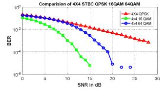
From the figure, it can be concluded that  $4 \times 4$  16-QAM gives better results compared to other modulation techniques when there are four transmit antennas and four receivers.
