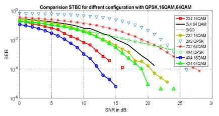
From the figure, the  $4\times4$  16-QAM gives better results ie., less BER when a stream of data is sent from transmitter to receiver. Therefore it can be concluded that if we use only single antenna for reception, the more will be the BER., if more number of antennas are used, BER will be reduced.
