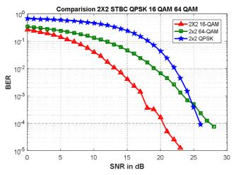
From the figure, it can be concluded that  $2 \times 2$  16-QAM gives better results compared to other modulation techniques when there are two transmit receivers.
