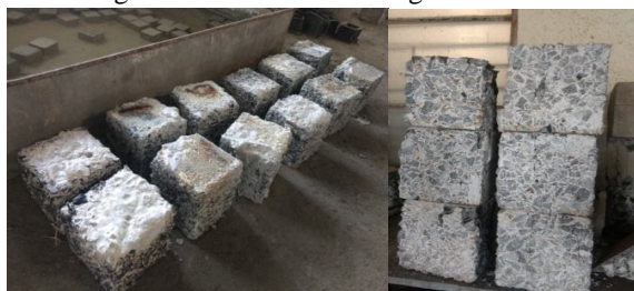
Fig 3.1 cubes after removing from acid tank
