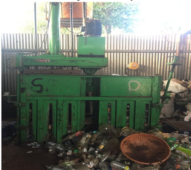
Fig -7 Punching Machine is used to punch the plastic bottles
