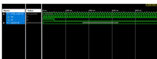
Fig:8 Simulation of modular LFSR of 64-bit
