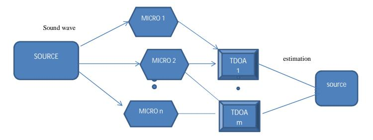
As seen in the block diagram, the signal sent by the source (speaker) is received by the microphones. It is then checked for synchrony on each of the pairs of microphones. For this purpose cross-correlation methods are used which gives an estimation of the time differences between the signals. One of the most commonly used cross-correlation methods is generalized cross-correlation with phase transform (GCC-PHAT).
