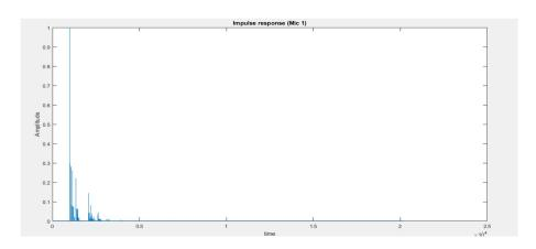
The wave generated with respect to the audio that is being given. A particular graph is generated from the given amplitude and time which shows the impulse response that is received in micropone 1
