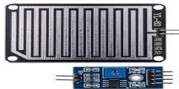
Fig. 4 Raindrop Sensor Plate and Module
